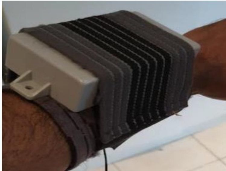
Figure 2: Fitting of WBAN on patient
