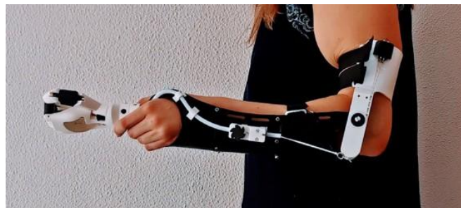
Figure 4: The bypass socket of the ADL arm
