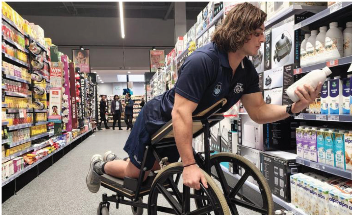
Pronemotion is a mobility solution for individuals with compromised independence. The Pronemotion was developed by students as part of the UCT Genesis Project in 2022 as a self-powered mobility vehicle that provides an alternative to the wheelchair. It is unique, cost effective and accessible. This MVP is currently being tested at one of Cape Town's top rehabilitation centres.
