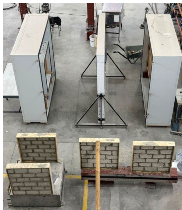
Figure 4: Guarded Hotbox set-up
